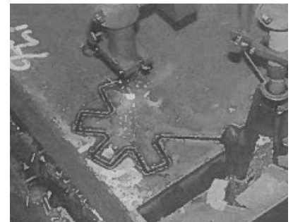
Figure 109: A flame cutter making a structural node for the British Museum Courtyard roof. Image source: [Barnes and Dickson, 2000]
