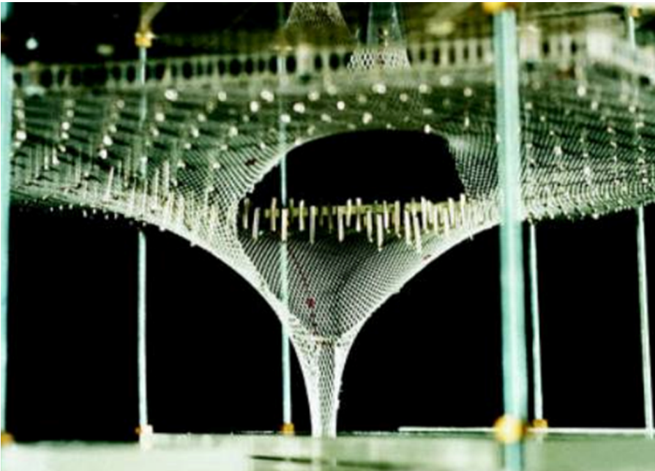
Figure 32: Frei Otto used physical models to aid in the form finding of the new train station in Stuttgart. The project is still in development after the death of Frei Otto. Image source: http://architecturehabitat.blogspot.dk
